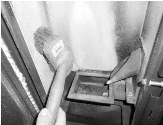
**Figure 117 – Nettoyage vermiculite**
