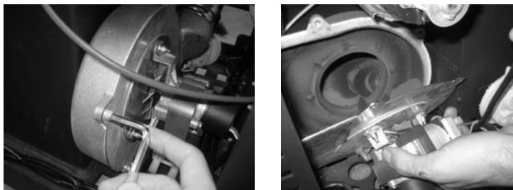
**Figure 143 – a) Remove the screws; b) Remove the extractor**
