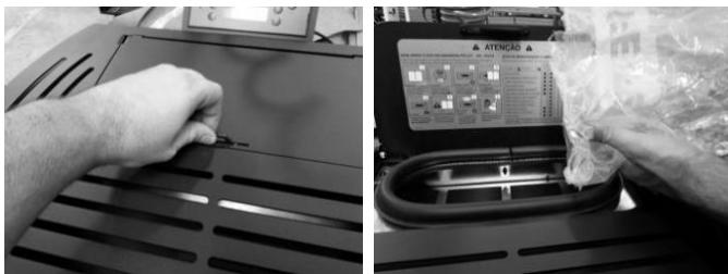
Figure 133 – Refilling the pellet reservoir
