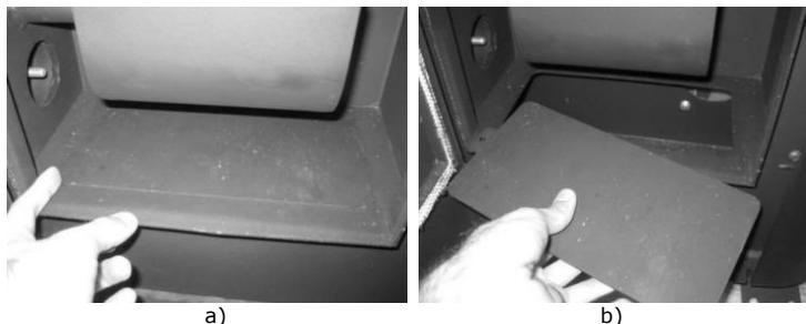
Figure 138 – Cleaning the Pellet Fire Unit's interior
