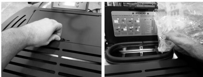
**Figure 135 – Refilling the pellet reservoir**
