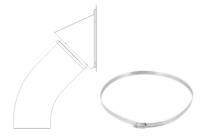
Figure 10 - Installation of the loading tube and metal clamp.
